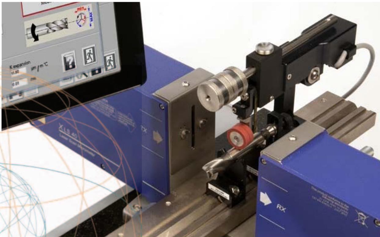
The SUPER-MECLAB+.T40 Bench Top Laser Micrometer is a high precision instrument for ultra-high accuracy diameter measurements of fluted part, with odd or even flutes. It is ideal for the off-line checking of
